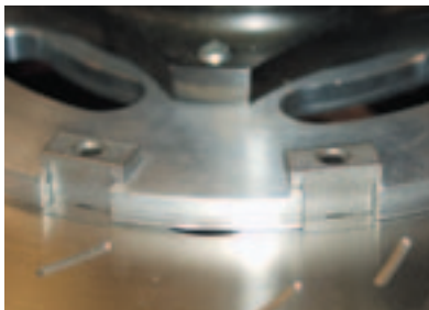
The T-bobbin hat design incorporates a single bolt through a "T" lock that attaches the rotor to the hat assembly. The rotor is clamped tight against the bobbin and the float is in the hat. This design has been the standard at Performance Friction.
